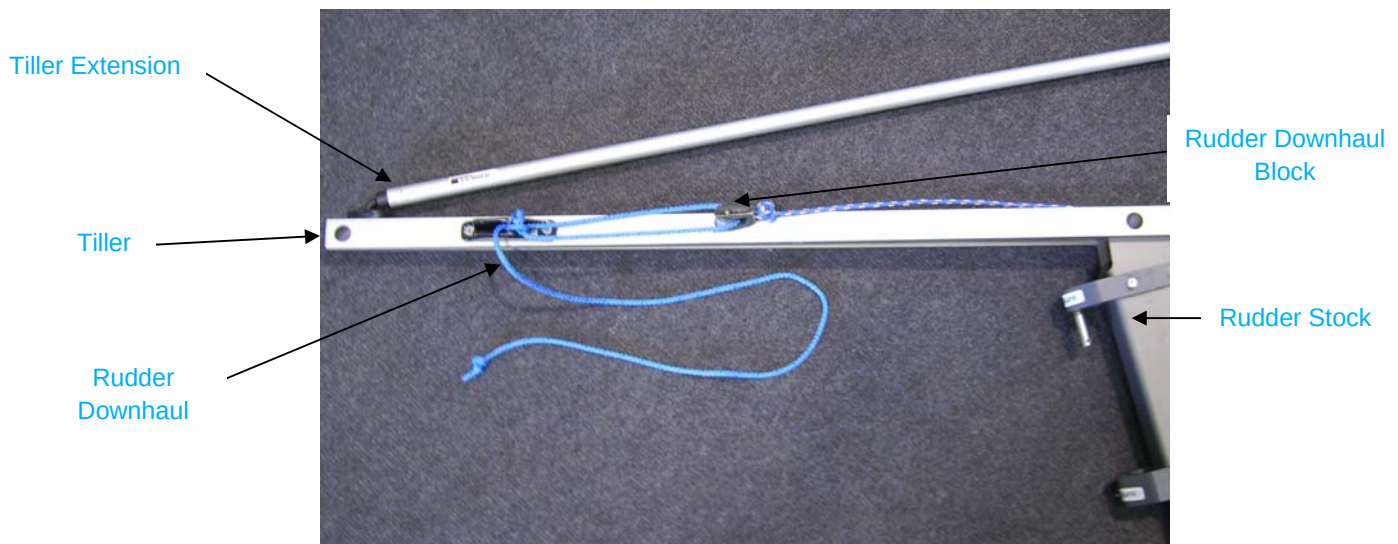
Picture 4.18 The Rudder Downhaul
